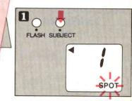
Press the shutter release button lightly, aiming at the image desired. Confirm that the "AF" indicator (green) in the viewfinder lights.
