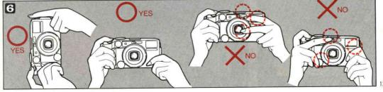
☑Gently press the shutter release button. If you press the button too quickly, the camera may shake, causing blurred pictures.
