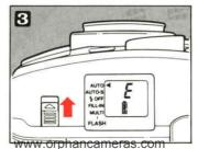
Battery power will be displayed in the LCD panel.
