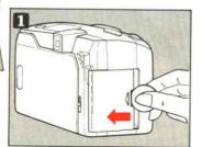
Two 3V lithium batteries (DL123A/CR123A)
